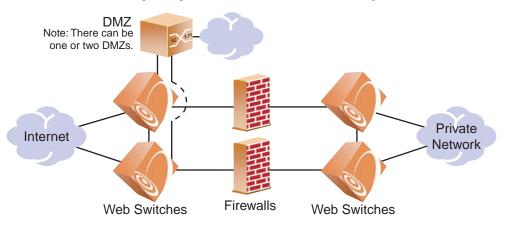
Figure 13-10 Typical Firewall Load-Balancing Topology with DMZ
